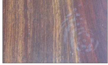
Prints mainly confined to one board and not adjacent boards. Does this suggest that the board or the drying of the sealer or coating on that board had an influence?
